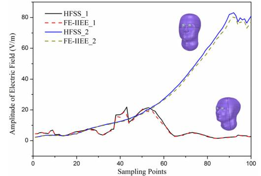
Fig. 5. Electric field amplitudes along two line segments obtained by the HFSS software and the FE-IIEE method. The first line segment is from the center of left ear to the center of right ear. The second line segment is from the center of the neck to the center of the top of the head model.
