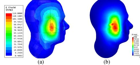
Fig. 4. Electric field amplitudes within the skin layer of the human head model obtained by (a) HFSS software and (b) FE-IIEE method.
