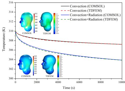
Fig. 6. 3-D temperature distributions at  $t = 10\,000$  s and the temporal temperatures at a randomly chosen observation point obtained by (a) COMSOL software and (b) TDFEM.
