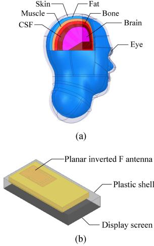
Fig. 2. (a) Head model. (b) Cell phone model.
