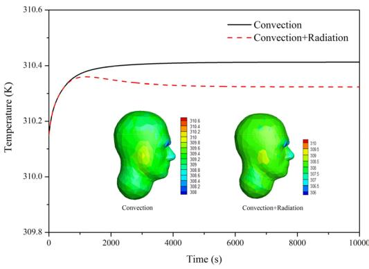
Fig. 7. 3-D temperature distributions at  $t = 6000$  s and the temporal temperatures at a randomly chosen observation point obtained by the proposed electromagnetic and thermal cosimulation method.
