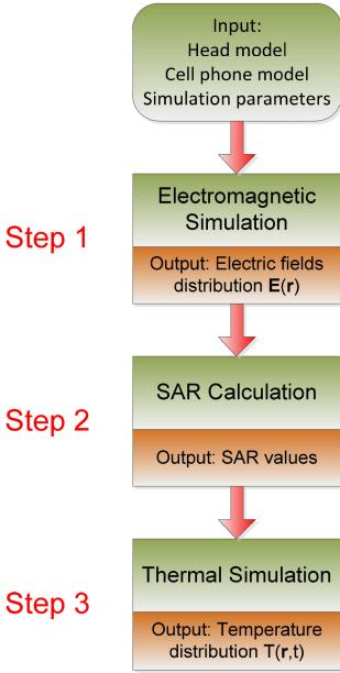
Fig. 1. Flow diagram for the electromagnetic-thermal analysis of human head exposed to cell phones.
