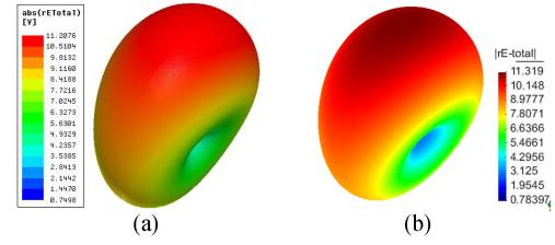
Fig. 3. Radiation pattern obtained by the (a) HFSS software and (b) FE-IIEE method.
