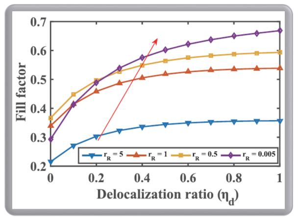
The saturation point of fill factor increases when the recombination rate decreases.
