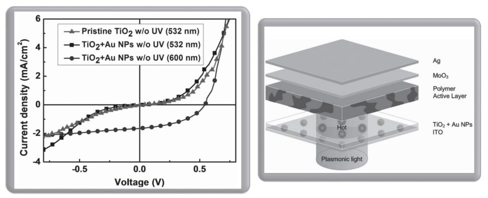
Pristine  $TiO_2$  buffer layer with many trap states induces effective extraction (reverse bias) and injection (forward bias) barriers and thus *S*-shaped current density-voltage (*J-V*) curve. On plasmonic resonance, plasmonically excited hot electrons are injected into  $TiO_2$  layer. The injected electrons eliminate the *S*-shaped *J-V* curve by trap filling and improve charge collection.
