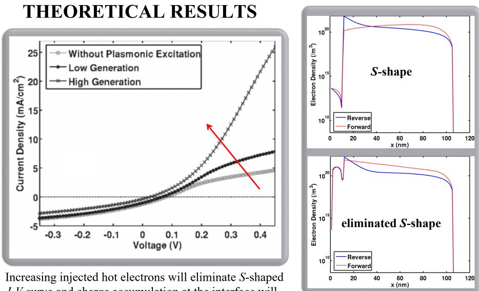
Increasing injected hot electrons will eliminate S-shaped J-V curve and charge accumulation at the interface will be improved.
