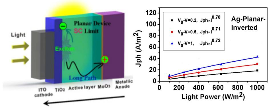
Light distribution mainly concentrates around cathode. Low-mobility holes travel a long distance. High-mobility electrons travel a short distance. Space charge limit (SCL) effect occurs.
