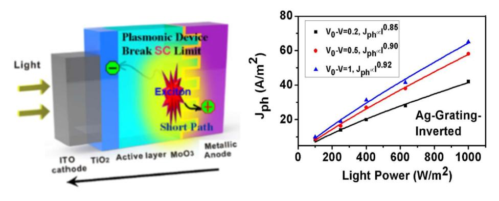
Light distribution concentrates around anode. Low-mobility holes travel a short distance. high-mobility electrons travel a long distance. SCL effect is broken by the plasmonic-electrical effect!
