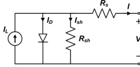
The PVSCs can be modeled by an equivalent circuit above. The current-voltage curve can be expressed by the Kirchoff's current law for the output current  $I$ .
