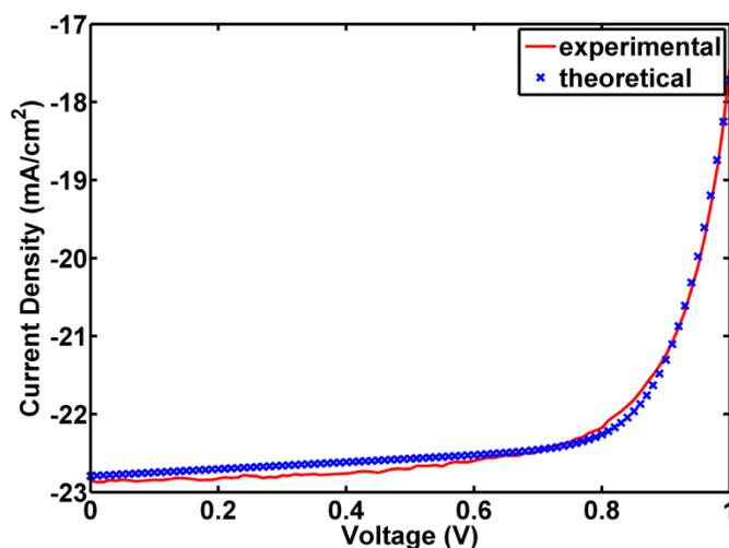
**Figure S3.** The theoretically fitted and experimentally measured  $J$ - $V$  characteristics for the high-performance perovskite solar cell. The device structure is given as: ITO/ NiO<sub>x</sub> (20 nm)/ CH<sub>3</sub>NH<sub>3</sub>PbI<sub>3</sub>(Cl) (300 nm)/ PCBM:C<sub>60</sub> mixture (50 nm)/ Bis-C<sub>60</sub> (10 nm)/ Ag (120 nm). The relative fitting error is 0.48%.
