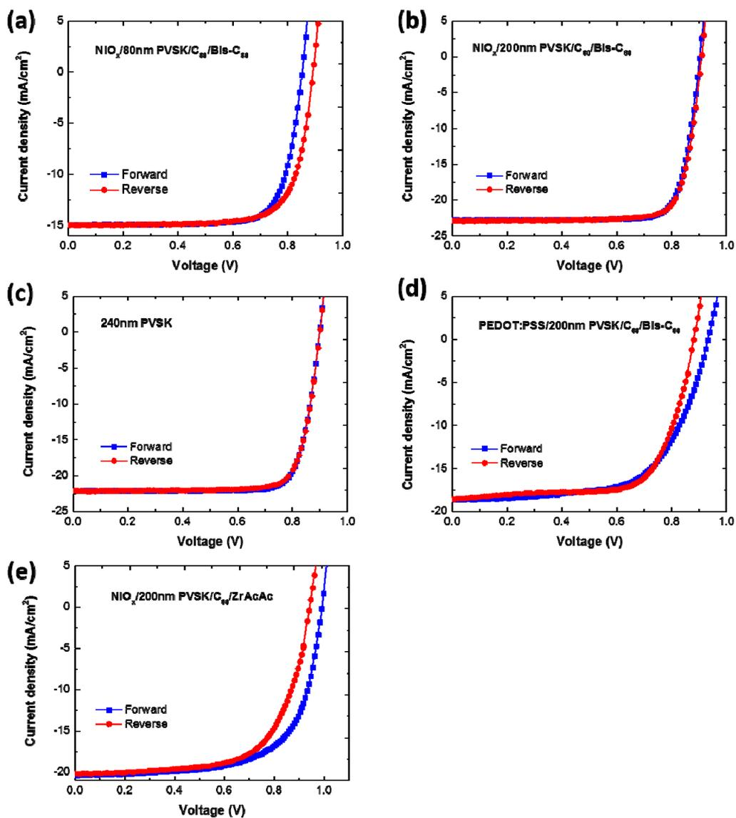
**Figure S1.** The  $J$ - $V$  characteristics for perovskite solar cells with different perovskite thickness (a, b, and c) and carrier transport layers (b, d, and e) measured under different scan directions.
