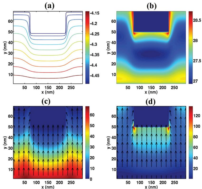
Figure S6: (Color online) The electrical results of the plasmonic OSC at the maximum power point. (a) equipotential lines (V); (b) recombination rate with the logarithmic scale ( $\text{m}^{-3}\text{s}^{-1}$ ); (c,d) electron and hole current densities ( $\text{A}/\text{m}^2$ ). The color and arrow denote the amplitude and direction of the currents.
