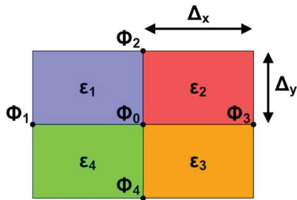
Figure S1: (Color online) The five-point stencil for the FDFD method.  $\Delta_x$  and  $\Delta_y$  are respectively the spatial steps along the  $x$  and  $y$  directions.  $\Phi = E_z$  for the TE polarization and  $\Phi = H_z$  for the TM polarization. Here,  $\epsilon = n_c^2$  is the relative permittivity in the discretized region and  $n_c$  is the complex refractive index of the optical material.
