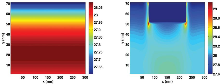
Figure S3: (Color online) The exciton generation rate of the standard OSC in the active layer.
