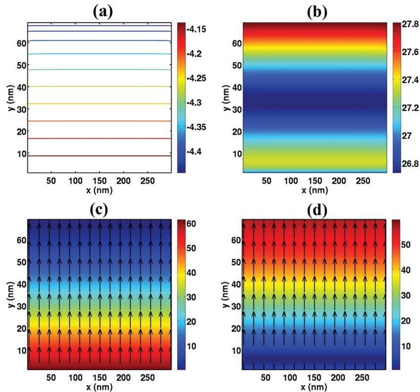
Figure S5: (Color online) The electrical results of the standard OSC at the maximum power point. (a) equipotential lines (V); (b) recombination rate with the logarithmic scale ( $\text{m}^{-3}\text{s}^{-1}$ ); (c,d) electron and hole current densities ( $\text{A}/\text{m}^2$ ). The color and arrow denote the amplitude and direction of the currents.
