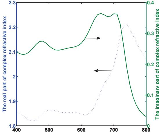
Figure S2: (Color online) The complex refractive index of the active polymer material. The active material is PBDTTT-C-T (poly{[4,8-bis-(2-ethyl-hexyl-thiophene-5-yl)-benzo[1,2-b:4,5-b']dithiophene-2,6-diyl]-alt-[2-(2'-ethyl-hexanoyl)-thieno[3,4-b]thiophen-4,6-diyl]}) and PC<sub>70</sub>BM ([6,6]-phenyl C<sub>71</sub>-butyric acid methyl ester) as donor and acceptor, respectively. (1:1.5, weight ratio in blend polymer.)
